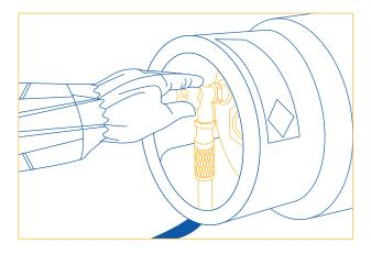
3. Unclip and remove the cylinder from forklift, using correct manual handling techniques (such as squatting or lowering the empty cylinder to the ground with one or two person lift as appropriate), and place in the designated location. Note: **All** cylinders must be stored upright, including empty cylinders.
